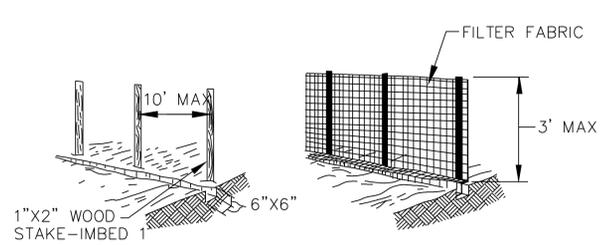
1. SET STAKE AND EXCAVATE A 6" X 6" TRENCH UPSLOPE ALONG THE LINE OF POSTS.
