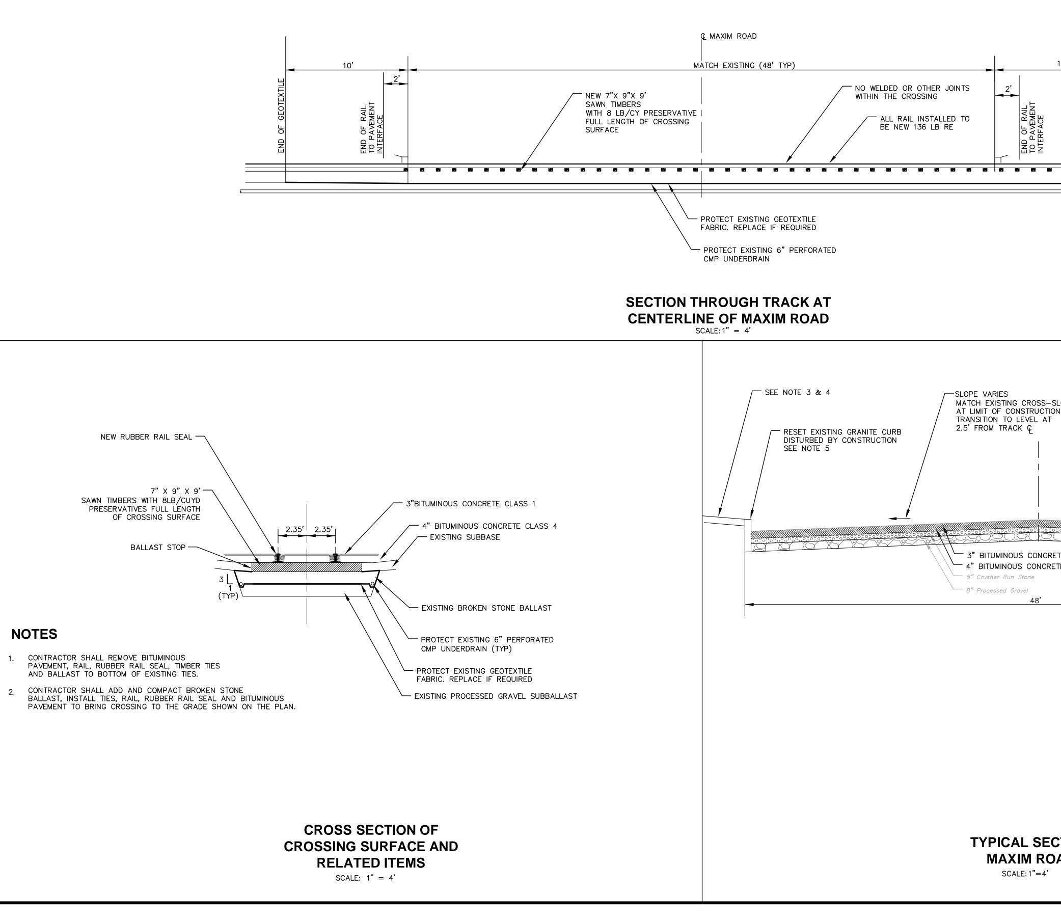
NOTE WELDED 136 RE RAIL TO EXTEND A MINIMUM OF 2 INSULATED JOINTS ON BOTH SIDES OF CROSSING
